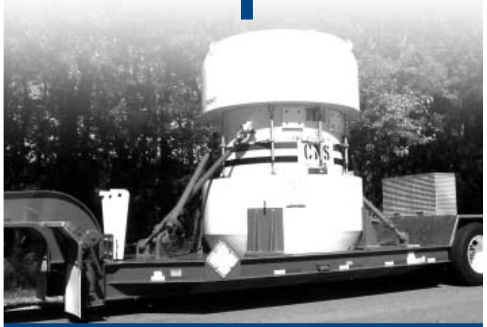
The U.S. Department of Energy will use this cask to ship remote-handled transuranic waste from a former weapons site in Columbus, Ohio to another facility for storage as part of a cleanup of the Ohio site. Photo by James Eide, Battelle.
