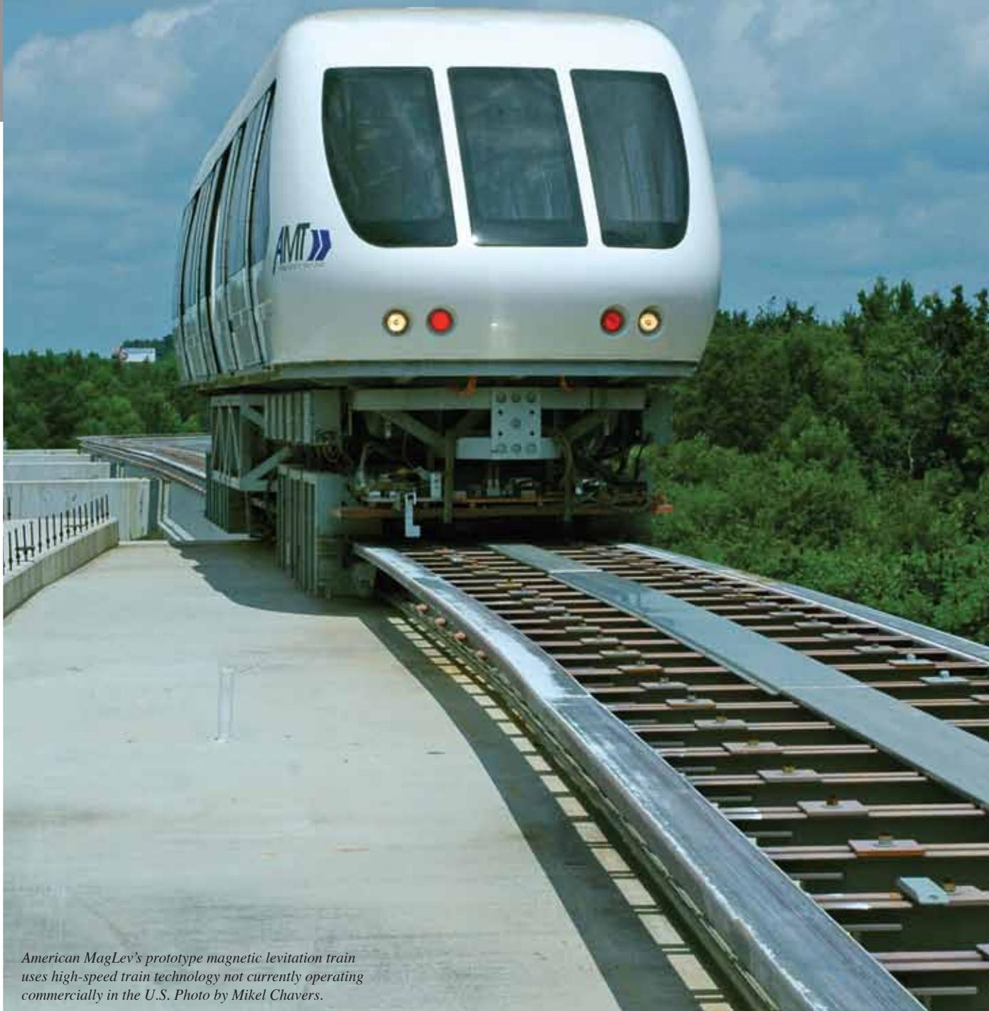
*American MagLev's prototype magnetic levitation train uses high-speed train technology not currently operating commercially in the U.S. Photo by Mikel Chavers.*
